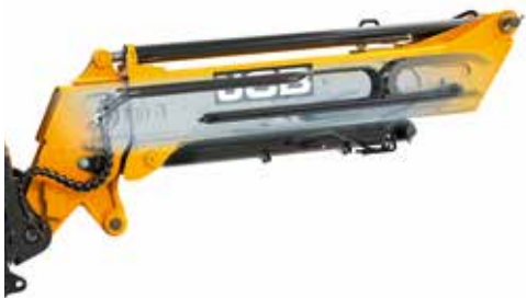
Hydraulic hoses are routed within the main boom structure to guard against damage.
