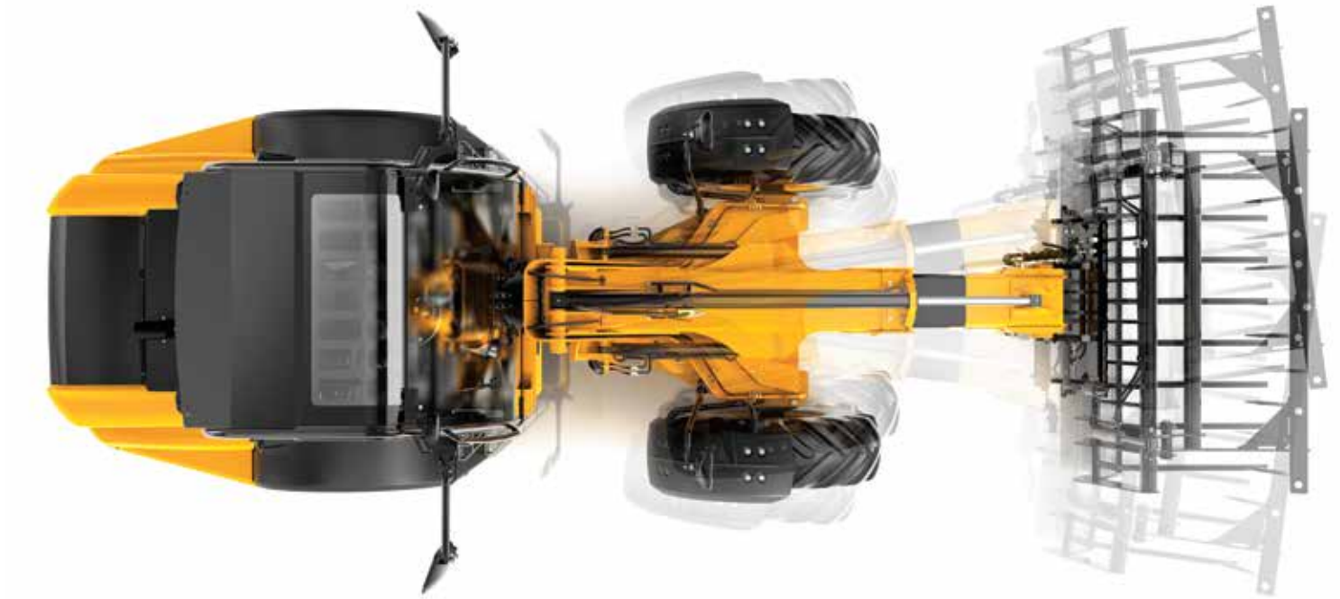
Articulated steering and a telescopic boom allow accurate positioning of loads.
